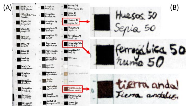
Figure 1. False RGB images ([605, 535, 430] nm) of laboratory samples in cotton paper. (A) Full pages; (B) Extracted minicubes.
