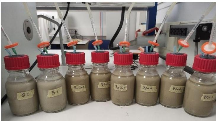
**Supplementary Figure S1.** Water-saturated bentonite microcosms of different treatments bubbling with N<sub>2</sub> to get anoxic conditions.
