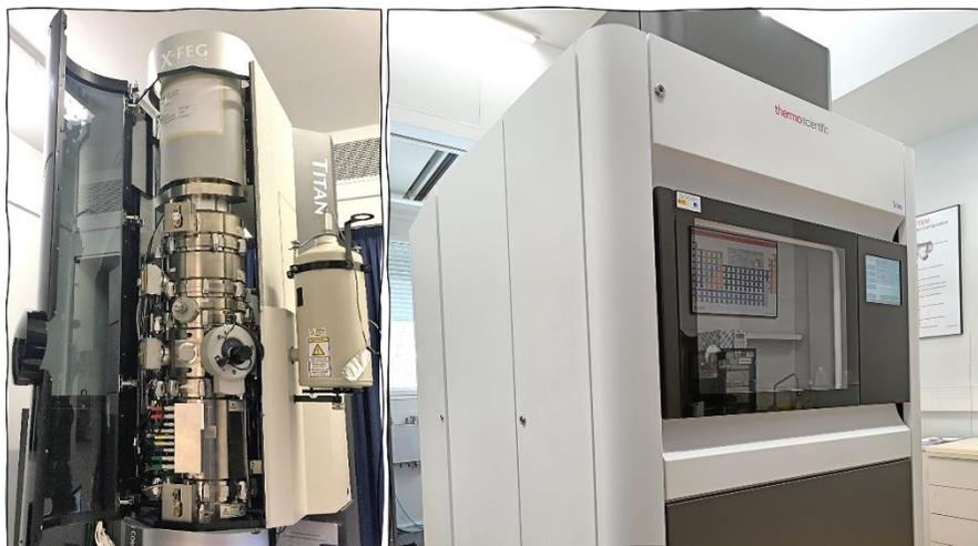
**Figure 4.** Ultra-high resolution transmission electron microscopes with high-angle annular dark-field (HAADF): FEI TITAN G2 (left) and Thermo Fisher Scientific TALOS F200X (right).
