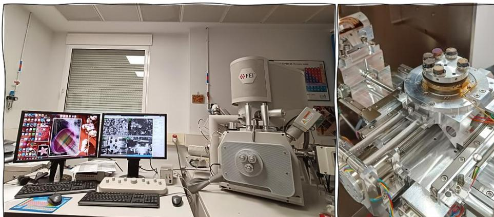
**Figure 5.** Environmental scanning electron microscopy (ESEM, FEG-ESEM QUEMSCAN 650F) (left) and copper disks on the holder of the variable pressure field emission scanning electron microscope (VP-FESEM, Zeiss SUPRA40VP) (right).
