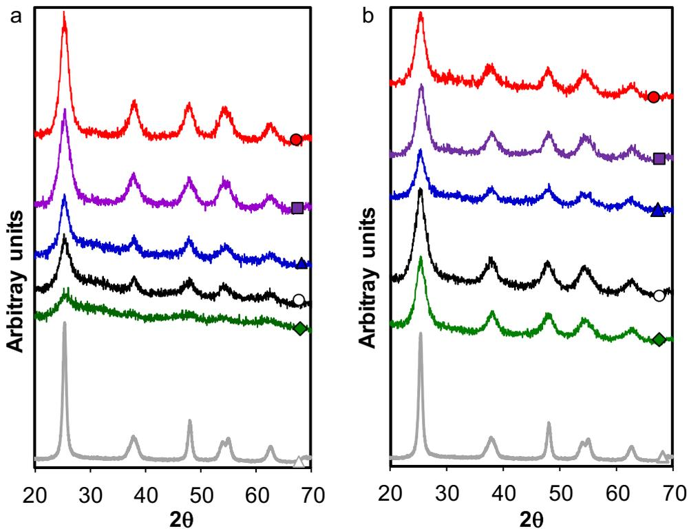
**Figure 4.** XRD patterns of a)  $\text{TiN}_x$  and b)  $\text{TiH}_x$  samples. x: 1 ( $\blacklozenge$ ), 2 ( $\circ$ ), 3 ( $\blacktriangle$ ), 4 ( $\blacksquare$ ) or 5 ( $\bullet$ ) regarding commercial  $\text{TiO}_2$  as reference material ( $\Delta$ )
