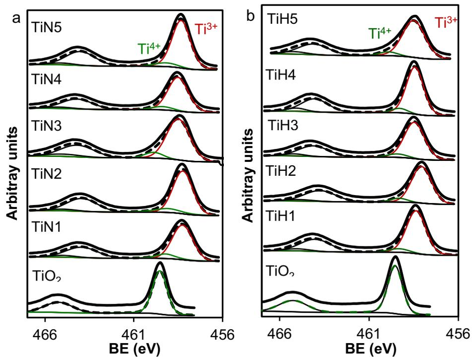
**Figure 3.** Ti2p region of XPS spectra for a) TiNx and b) TiHx samples.
