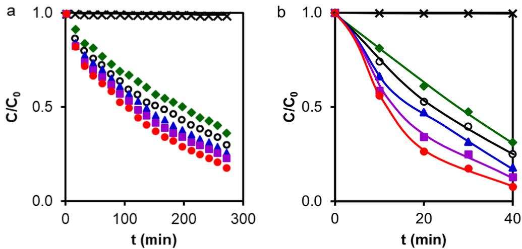
**Figure 8.** Kinetic of Orange G photocatalytic degradation using a) TiNx and b) TiHx samples in comparison with white  $TiO_2$  (x). x: 1 (◆), 2 (○), 3 (▲), 4 (■) or 5 (●).
