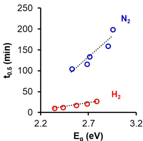
**Figure 9.** Relationship between the time needed to achieve the 50 % of Orange G degradation ( $t_{0.5}$ ) and the photocatalyst band gap. TiHx ( $\circ$ ), TiNx ( $\square$ ) and TiO<sub>2</sub> ( $\Delta$ ).
