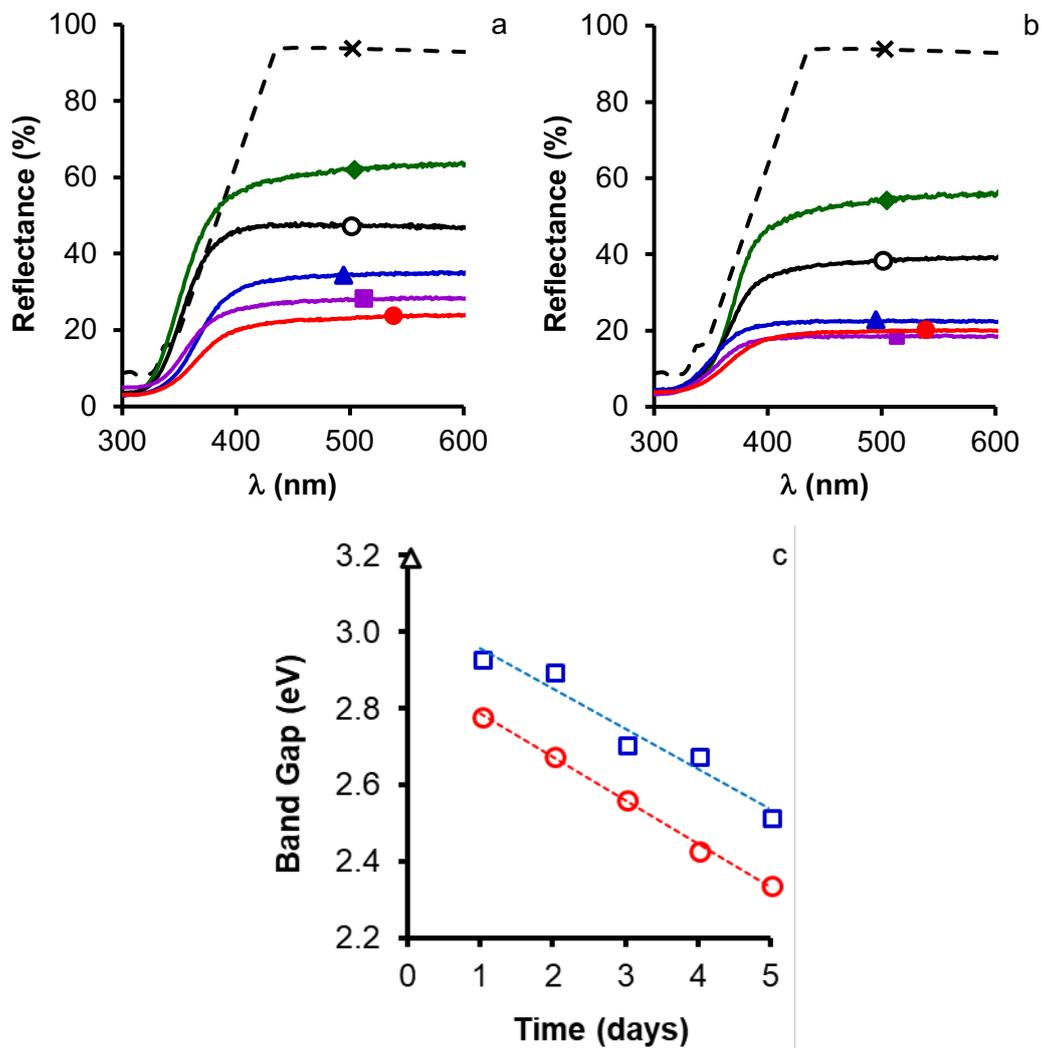
**Figure 2.** Diffuse reflectance spectra of a)  $TiNx$  and b)  $TiHx$  samples in comparison with white  $TiO_2$  (x) as reference, being x: 1 ( $\blacklozenge$ ), 2 ( $\circ$ ), 3 ( $\blacktriangle$ ), 4 ( $\blacksquare$ ) or 5 ( $\bullet$ ); c) Band gap of  $TiNx$  ( $\square$ ),  $TiHx$  ( $\circ$ ) and white  $TiO_2$  ( $\Delta$ ).
