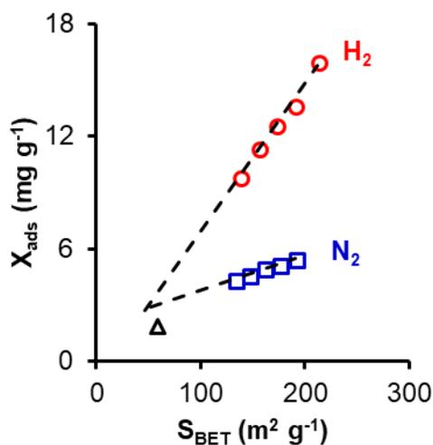
**Figure 7.** Orange G adsorption capacity of samples as a function of surface area. TiHx ( $\circ$ ), TiNx ( $\square$ ) and TiO<sub>2</sub> ( $\Delta$ ).
