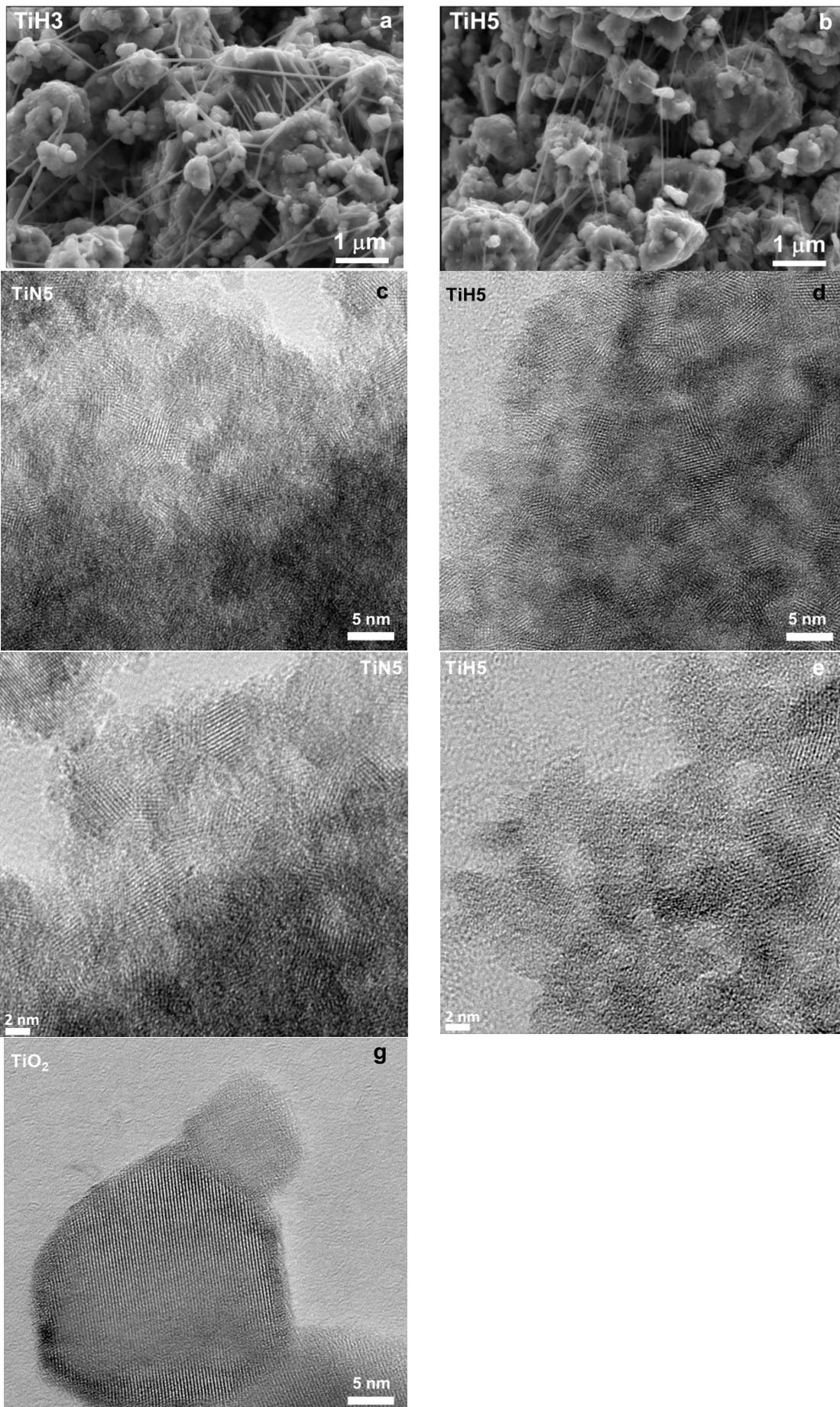
**Figure 5.** Characteristic SEM (a,b) and TEM (c-g) images of the black titania
