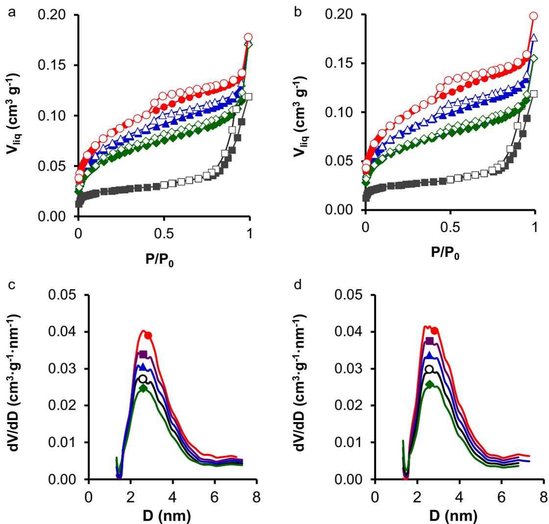
**Figure 6.** N<sub>2</sub>-isotherms and pore size distributions for TiN<sub>x</sub> (a,c) and TiH<sub>x</sub> (b,d) samples in comparison with TiO<sub>2</sub> (□). x: 1 (◆), 2 (○), 3 (▲), 4 (■) or 5 (●).
