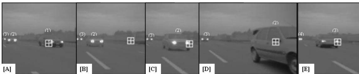
**Figure 8.2.** Multiple cars overtaking on a highway on a cloudy day. Number labels on the top of the cars are added to clarify the process. The reliable position is marked automatically by the system in the figures using a white cross.
