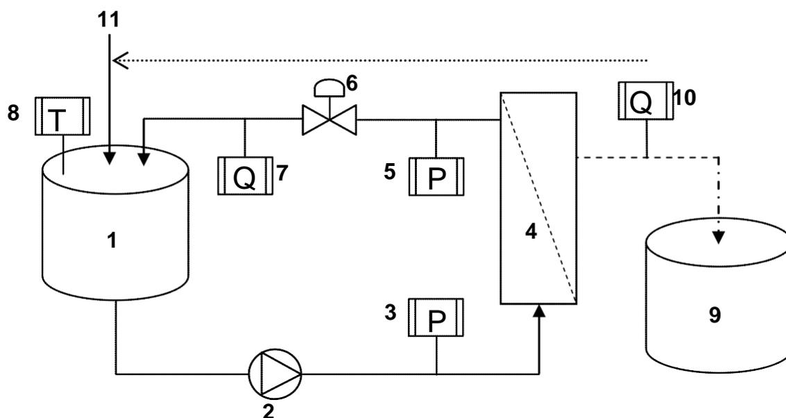
Fig. 1. Process flow diagram: Feed tank (1), pump (2), pressure gauge (3, 5), membrane module (4), valve (6), retentate flow meter (7), temperature probe (8), permeate tank (9), permeate flow meter (10), feed (11).
