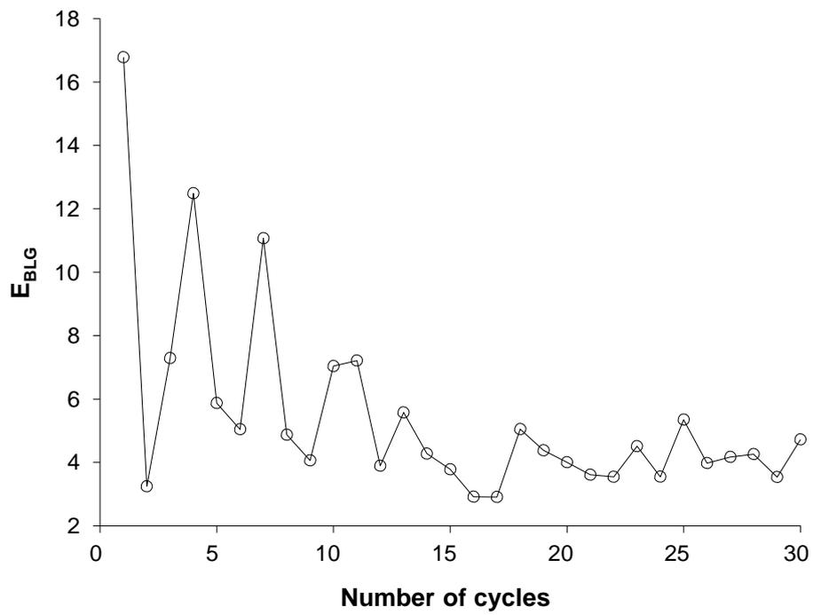
Fig. 9. Efficiency on the final separation of BSA (a) and BLG (b) as a function of the number of cycles for membrane A.
