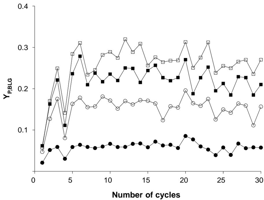
Fig. 7. Evolution of the permeate yield of BSA (a) and BLG (b) with the number of cycles for membrane A. Series represent diafiltration times of 1 (●), 2 (○), 3 (■) and 4 h (□).
