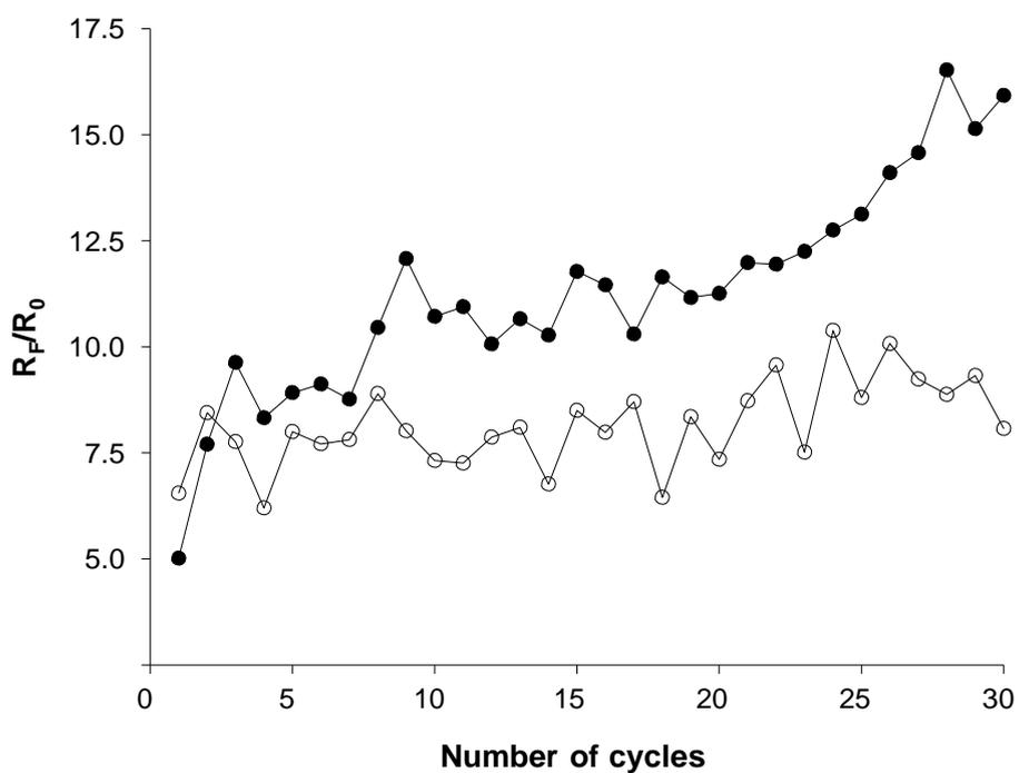
Fig. 4. Evolution of the normalized fouling resistance with the number of cycles for membrane A (○) and B (●).
