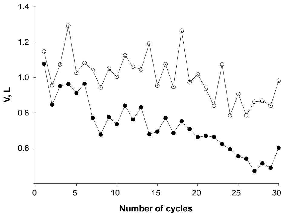
Fig. 2. Final permeate volume as a function of the number of cycles for membrane A (○) and B (●).
