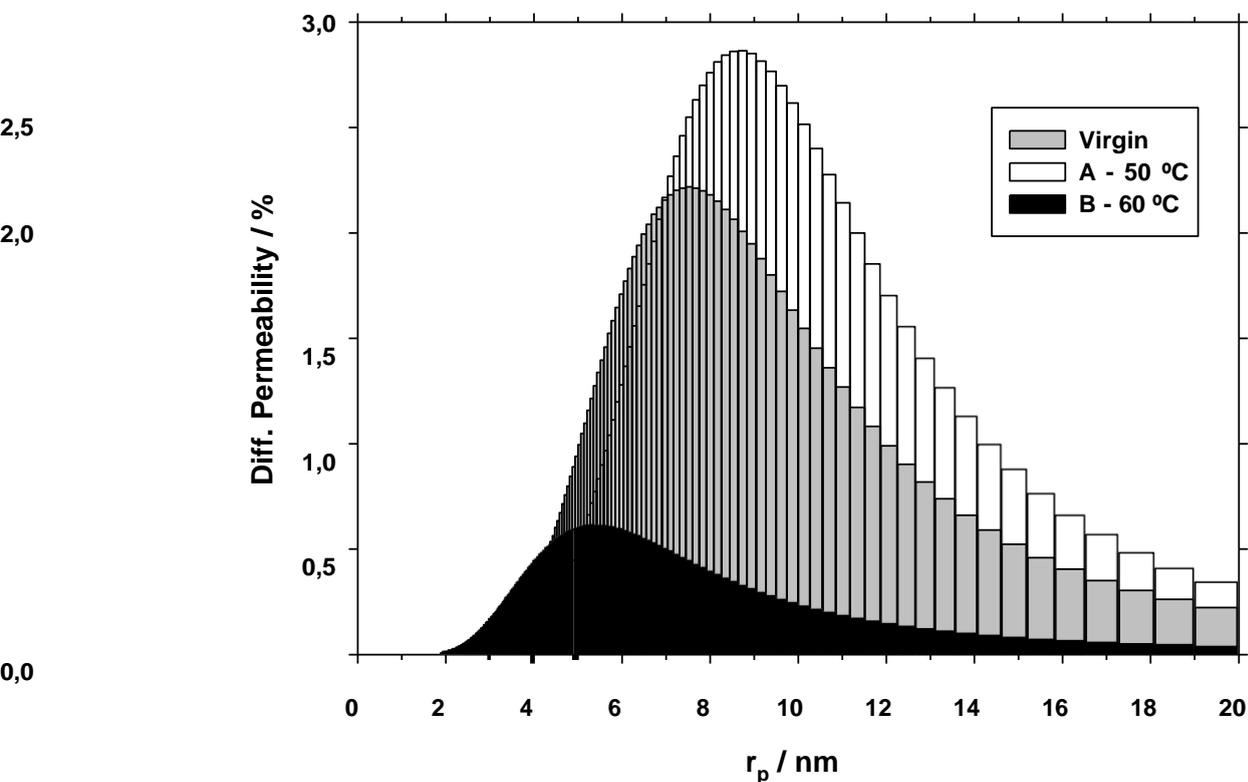
Fig. 10. Pore size distribution from permeability data for the virgin membrane, membrane A (50 °C) and membrane B (60 °C).
