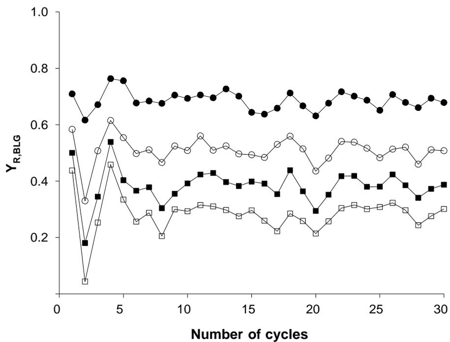
Fig. 6. Evolution of the retentate yield of BSA (a) and BLG (b) with the number of cycles for membrane A. Series represent diafiltration times of 1 h (●), 2 h (○), 3 h (■) and 4 h (□).
