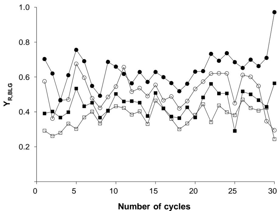
Fig. 8. Evolution of the retentate yield of BSA (a) and BLG (b) with the number of cycles for membrane B. Series represent diafiltration times of 1 (●), 2 (○), 3 (■) and 4 h (□).
