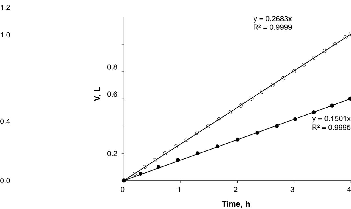
Fig. 3. Time evolution of the permeate volume for 1 (○) and 30 (●) operational cycles for membrane A (a) and B (b).
