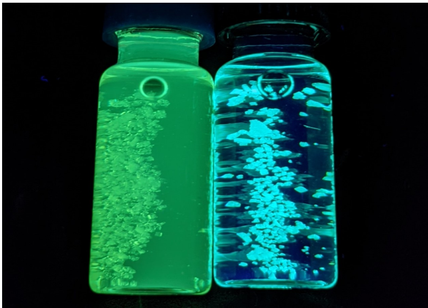
Figure S21. Photograph of vials illuminated at 365 nm containing PyC-β-CD-HF kept in the mother liquor (left), and fresh MeOH (right)
