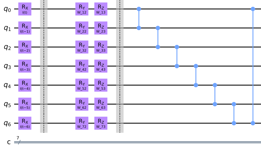
Figure 7.9: Example of a 7-qubit VQC with the structure used in the experiments. Left: encoding layer; middle: variational gates; right: entanglement CNOT gates organized in a ring.
