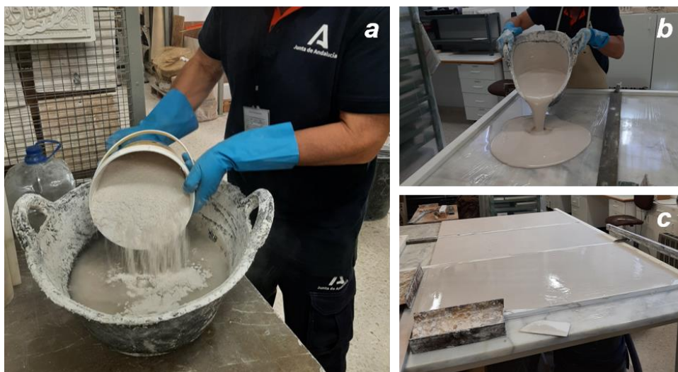
Figure A.4. Preparation of the gypsum plaster mock-ups used for the assessment of the consolidation efficacy of the prepared fluorescent nano-bassanite consolidant ethanolic suspensions. These specimens were prepared and cured at the plasterwork workshop of the Council of the Alhambra and Generalife. a) Mixing of bassanite with water; b) Pouring of the fresh paste into the mold; c) Final plaster board.
