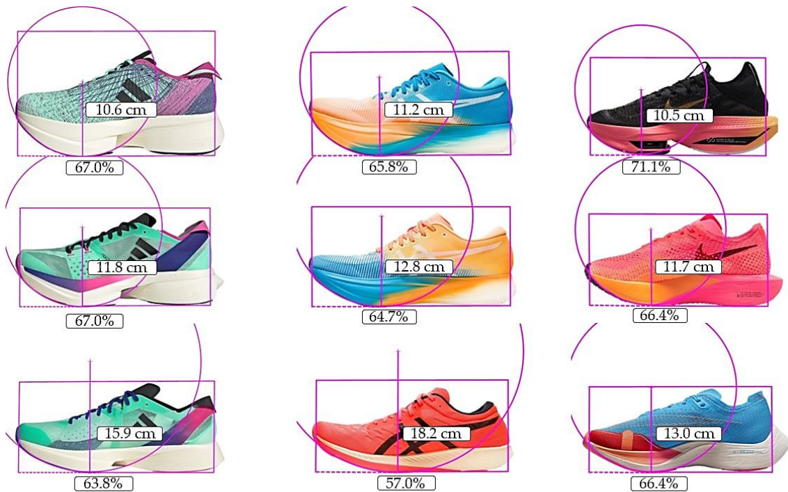
Figure 3. Rocker axis position (i.e., the starting point of the forefoot upward curvature) and rocker radius of current footwear models of different brands with different stack heights. The measures were performed with the Kinovea free-access software using a sagittal image of each model placed in the same position. The rocker axis was placed at the center of the rocker radius circle and calculated by the relative position to the total length (i.e., 28 cm for all models). The rocker radius indicates the degree of the upward forefoot curvature of the sole (i.e., a greater rocker radius indicates a lower upward curvature). (TOP): Adidas Adizero Prime X Strung (50 mm, 67%, 10.6 cm), (MIDDLE): Adidas Adizero Pro 3.0 (40 mm, 67%, 11.8 cm), (BOTTOM): Adidas Adizero Takumi Sen 9 (33 mm, 63.8%, 15.9 cm), (TOP): Asics Metaspeed Sky+ (39 mm, 65.8%, 11.2 cm), (MIDDLE): Asics Metaspeed Edge+ (39 mm, 64.7%, 12.8 cm), (BOTTOM): Asics Metaracer Tokyo (24 mm, 57%, 18.2 cm), (TOP): Nike Air Zoom Alphafly Next% (39 mm, 71.1%, 10.5 cm), (MIDDLE): Nike ZoomX Vaporfly Next% 3 (40 mm, 66.4%, 11.7 cm), (BOTTOM): Nike ZoomX Vaporfly NEXT% 2 (39 mm, 66.4%, 13.0 cm). Note that the rocker radius is an approximation.
