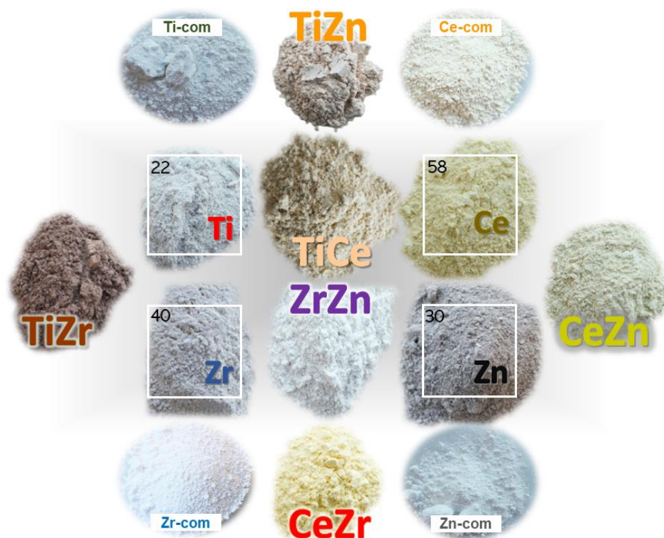
Figure 4.1. Photographs of semiconductor nanoparticles synthesized in monometallic and mixed phases. The corresponding commercial oxides are shown in the corner for comparison.
