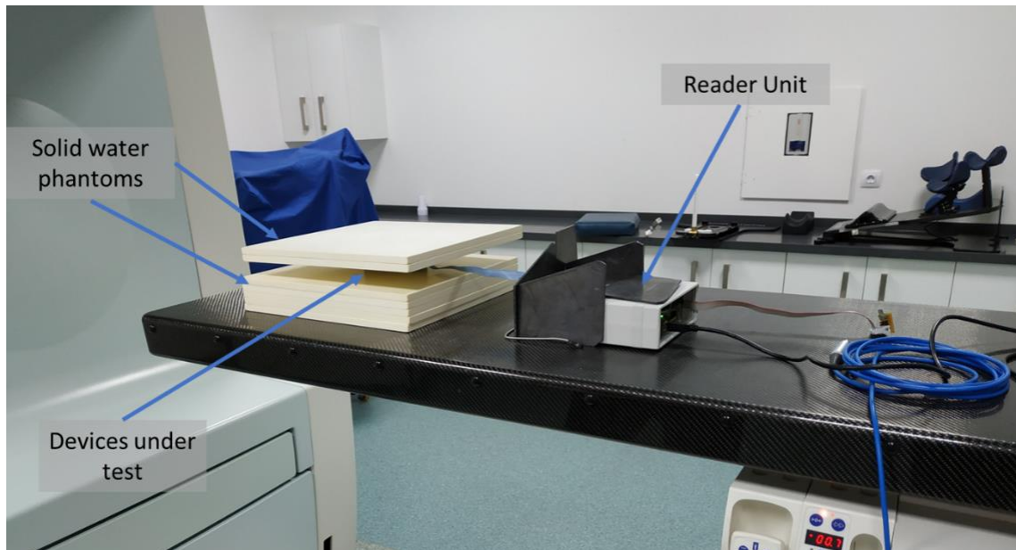
Figure 1. Experimental setup for the dosimetric characterization of the photodiode radiation response. Solid water layers are shown under and over the box containing the devices under test.
