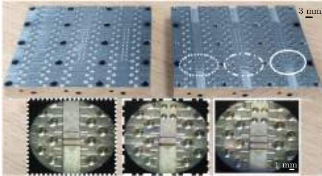
Fig. 16. Forming layers of the manufactured prototype and details under microscope.
