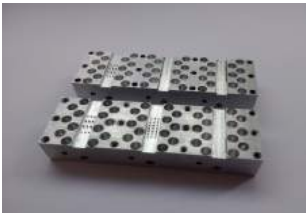
FIGURE 10: CNC milling manufactured prototype.
