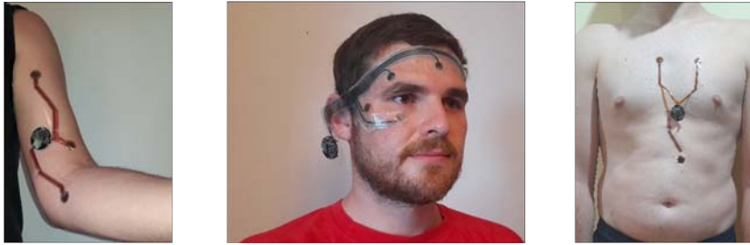
Figure 8.7: Position of electrodes in real case uses. (a) EMG acquisition. (b) EOG acquisition. (c) ECG acquisition.
