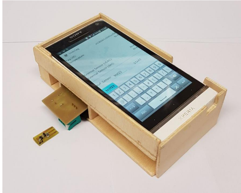
Figure 6. Experimental setup for NFC measurements
