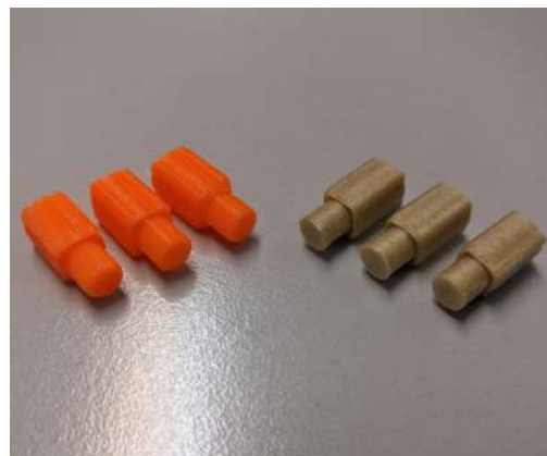
(c) Detail of the printed buttons. First tests: left (orange), second batch: right (brown).
