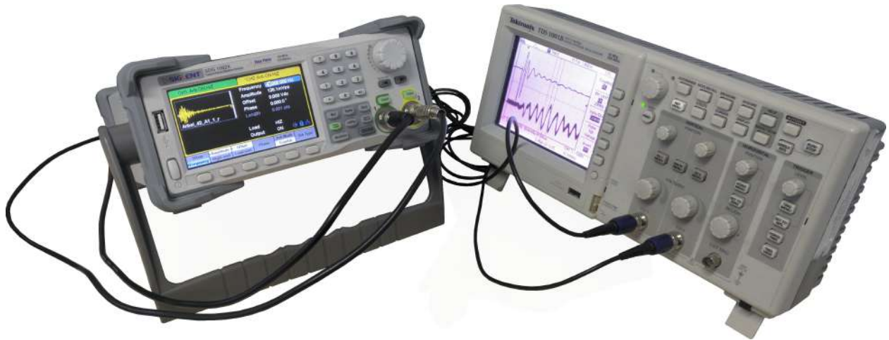
Figure F.10 – Siglent SDG1062X outputting emitter/receiver signals, and visualization with a Tektronix TDS1001B oscilloscope on GranaSat’s laboratory. Both devices are directly connected one another. The arbitrary generator is configured for a high-impedance (Hi-Z) load.
