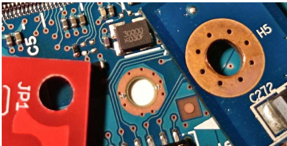
Figure 5.29 – Different types of PCB mounting holes. Credits: [162]. Left: not plated, without head landing or vias, but with copper clearance. Middle and right: grounded, non-plated, with copper head landing and vias.
