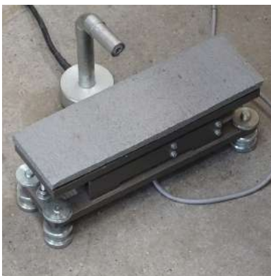
(g) PLG's microphone and load cell.
