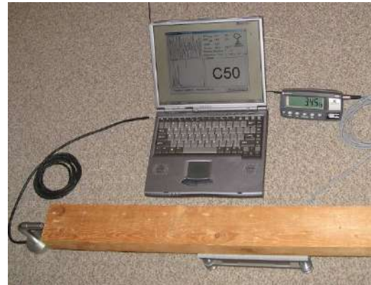
(f) Fakopp PLG during measurement [54].
