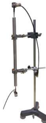
(e) Fakopp testing bar in a lab stand.
