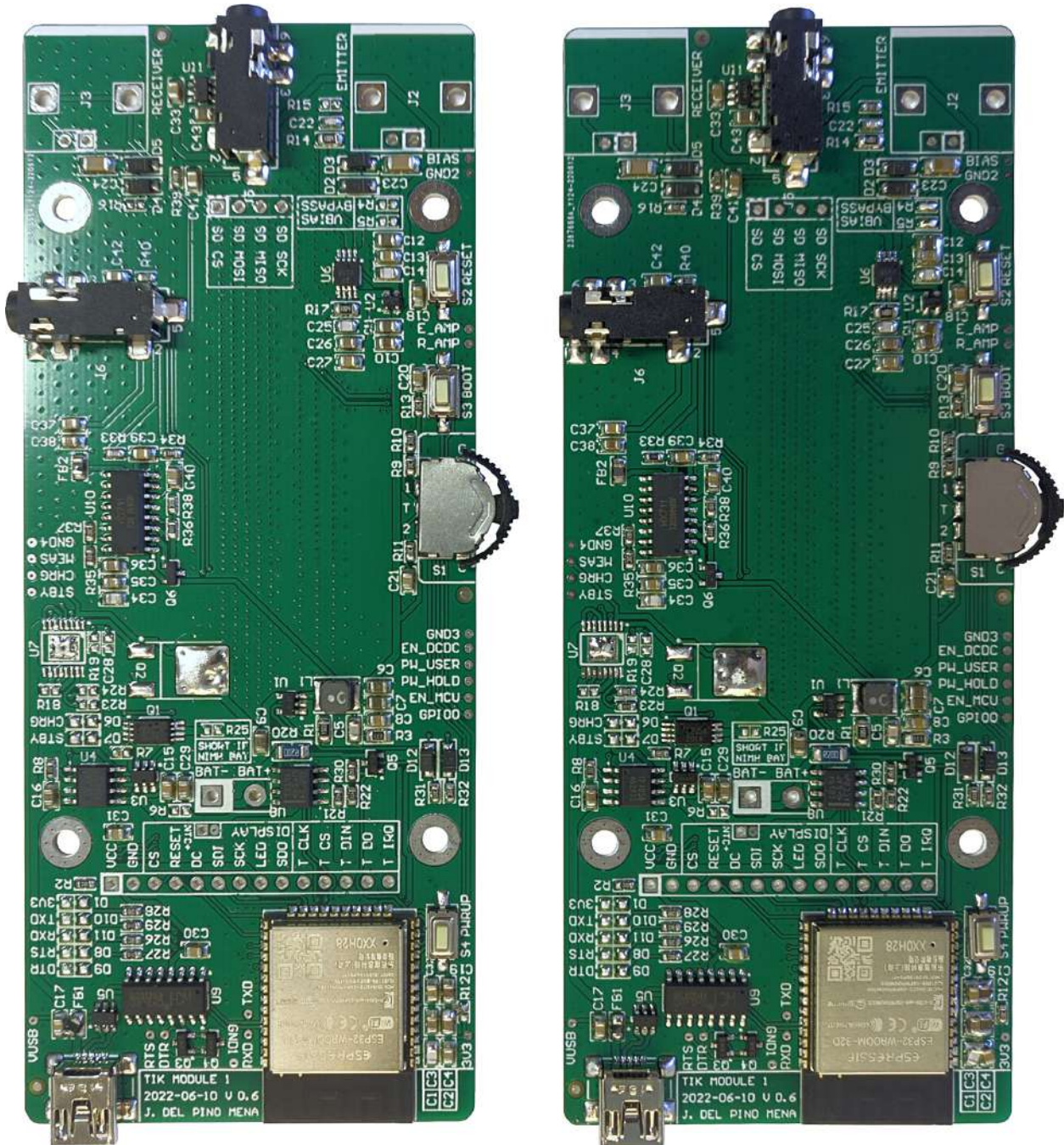
Figure 6.10 – The two PCBs after being reflow-soldered in the oven, with solder defects.
