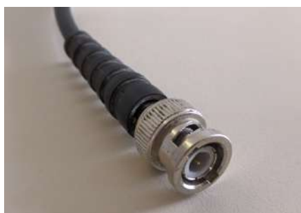
(e) Detail of the probes' male BNC connector.
