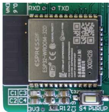
(a) Detail of the ESP32 after moving components and removing part of the solder with solder wick.
