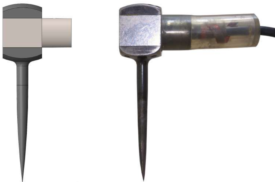
Figure 2.6 – Comparison of the profile of a real probe with the 3D model.
