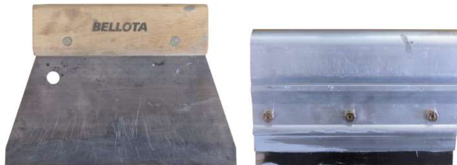
(c) Spatulas used to spread the solder paste on the stencil.
