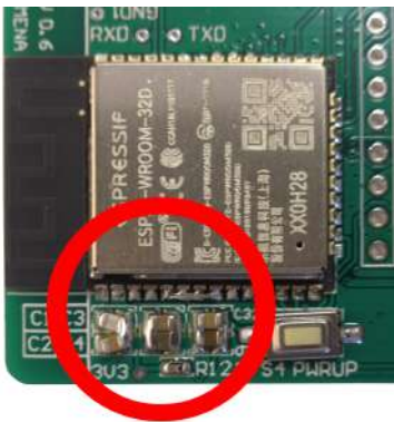
(d) Detail of the ESP32 and its bypass capacitors.
