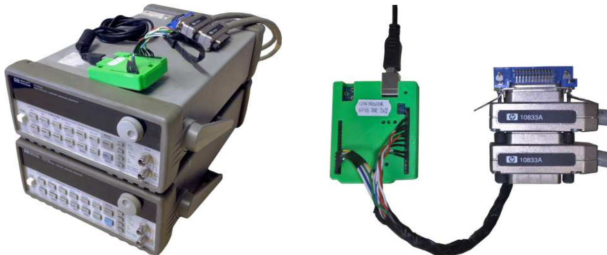
(a) Both HP33120A generators with the mediator on top.
