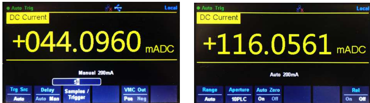
(a) LCD-only average power consumption measured with a Siglent SDM3065X digital multimeter.
