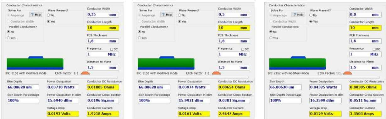
(c) Conductor characteristics of 0.35 mm width traces. (d) Conductor characteristics of 0.5 mm width traces. (e) Conductor characteristics of 0.8 mm width traces.
