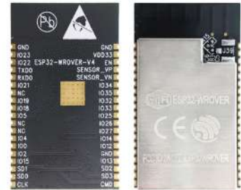
(f) Espressif ESP32-WROVER-x series package. Extracted from: [96].
