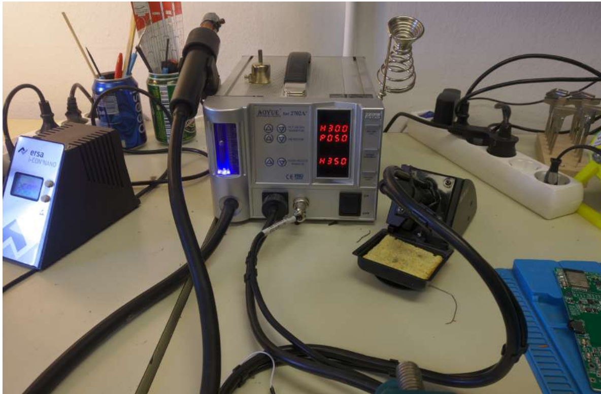
(a) The AOYUE Int 2702A+ soldering station at GranaSat.
