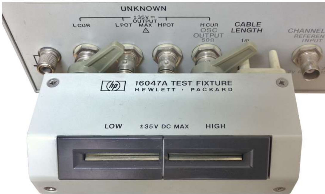
Figure F.17 – Detail of the 16047A test fixture and HP4192A UNKNOWN port.
