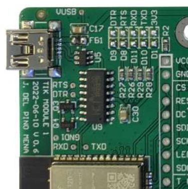
(b) Detail of the USB circuit after repositioning the ferrite bead.
