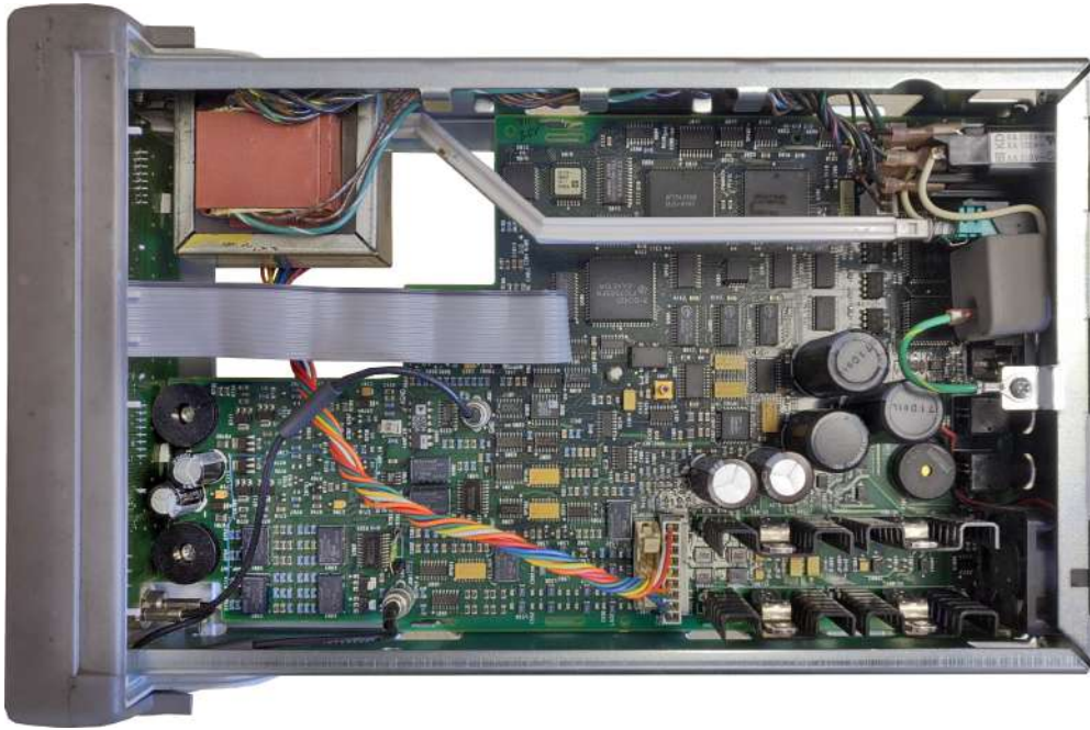
Figure F.5 – Photo of the internals of the HP33120A.
