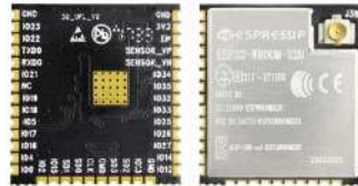
(e) Espressif ESP32-WROOM-32U. Extracted from: [95].
