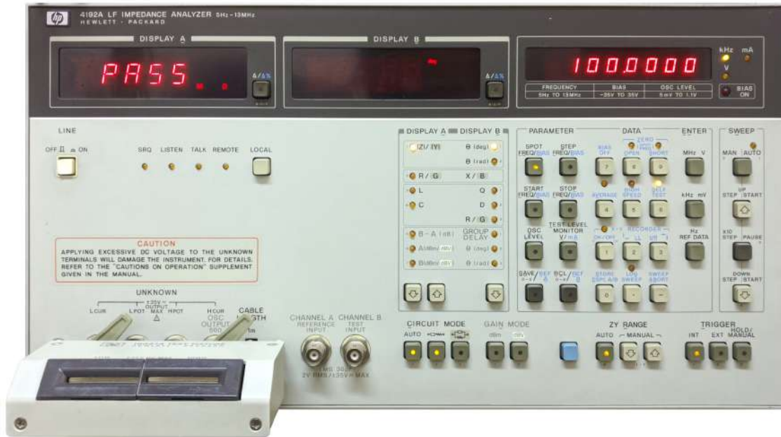
Figure F.16 – Front panel of the HP4192A LF impedance analyzer in the L-4 laboratory of the Faculty of Sciences; with the 16047A test fixture coupled.
