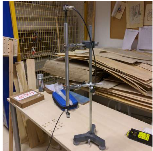
(d) Fakopp validation bar. Vertical mounting supported by lab stand.
