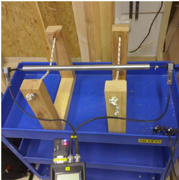
(c) Fakopp validation bar. Horizontal mounting suspended on ropes.
