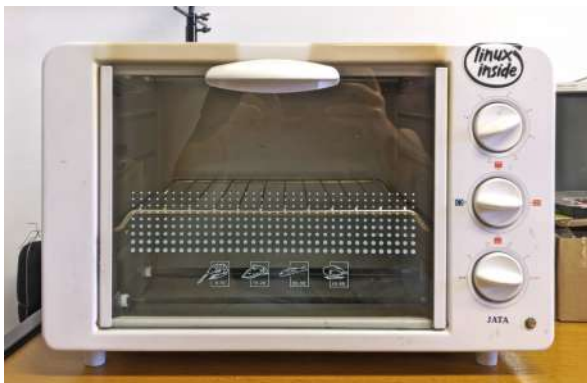
(a) Oven used for reflow soldering at GranaSat's.
