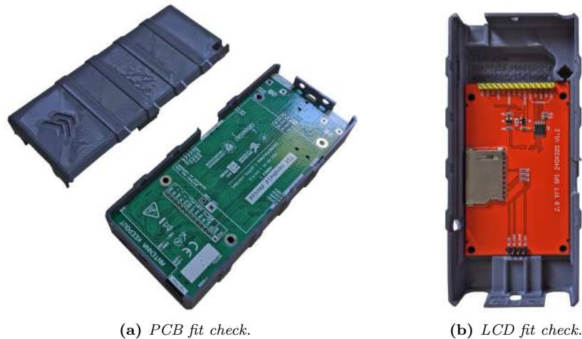
Figure 6.19 – Checking that the PCB and display module fit correctly into the 3D printed parts.
