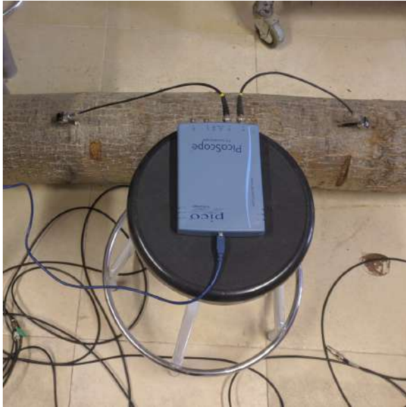
(a) Measurements in log with the Picoscope 4424.
