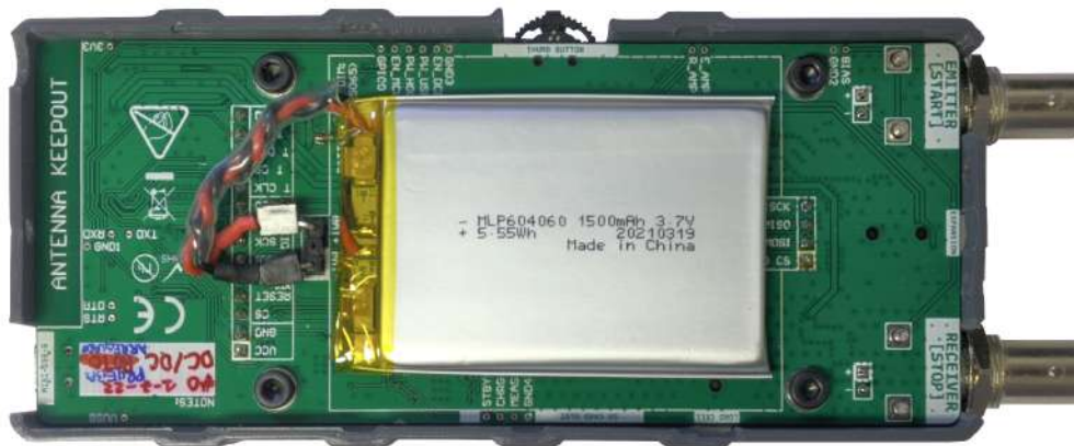
Figure 6.20 – PCB screwed to the top cover, with battery.
