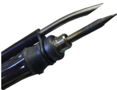
(b) Detail of the soldering iron with fume absorber.
