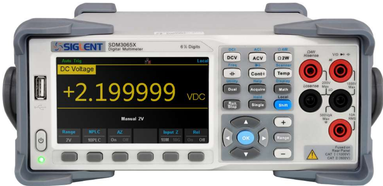
Figure F.18 – Front panel of the SDM3065X digital multimeter. Extracted from: [193].
