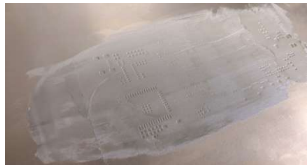
(e) Stencil with solder paste spread.
