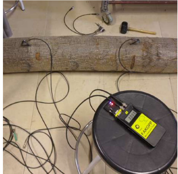
(b) Measurements in log with the Fakopp Microsecond Timer.
