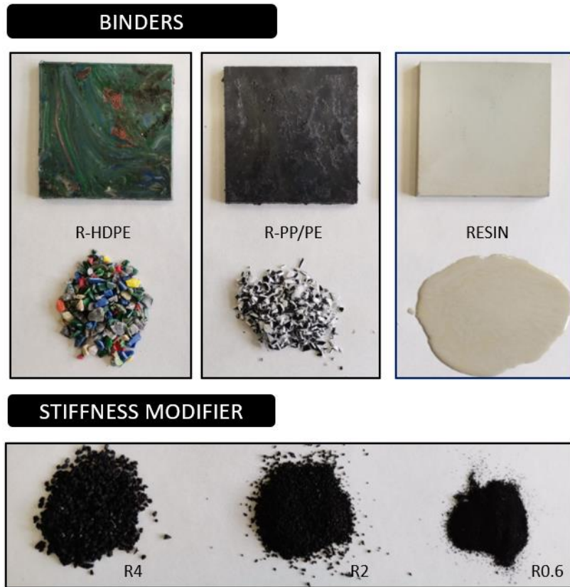
Figure 2. Visual appearance of the materials used for the manufacturing of sustainable pads.
