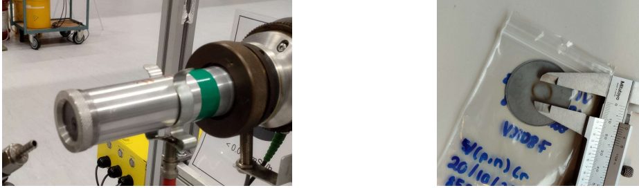
(a) Real picture of the ^{51}\text{V} target placed in the beamline with the fixing system. The proton beam air flow is illustrated. (b) ^{51}\text{V} target foil with a mark left by the proton beam.
