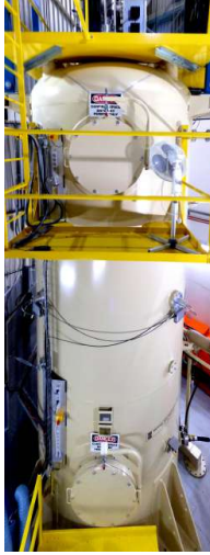
(a) Vertical 3.5 tandem accelerator [116].
