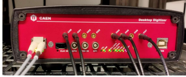
Figure 3.10. Picture of the CAEN digitizer DT5730 used in our experiment.
