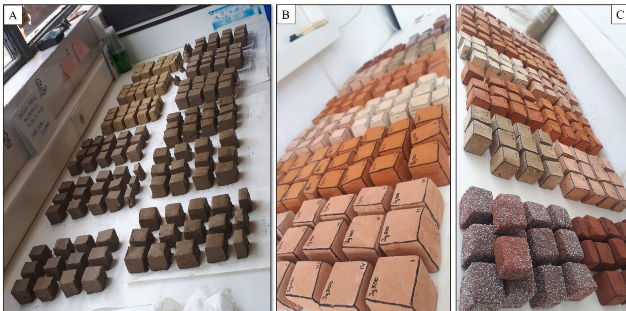
Fig. 1. Photograph of the bricks studied in this work. A) Unfired bricks made from raw materials from Jun and Guadix with and without household glass; B-C) General view of fired bricks with and without household glass.
