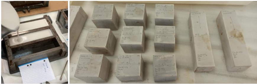
Figure 1. Left) Filling of molds. Right) Cubic and prismatic lime-based grout test specimens.
