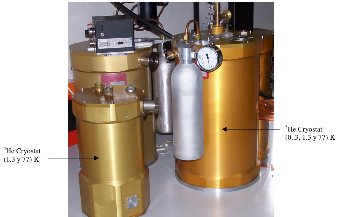
Figure (4c). Several ^4\text{He} and ^3\text{He} Cryostats for use in the Laboratory
