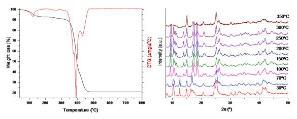
Fig. 2. TGA/DTG curves of Zn-URJC-8 (left). b) Temperature dependence PXRD patterns (right).
