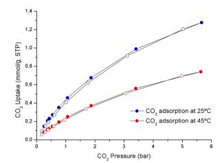
Fig. 3.  $\rm CO_2$  adsorption-desorption isotherms of Zn-URJC-8 at 25 and 45  $^\circ \rm C.$
