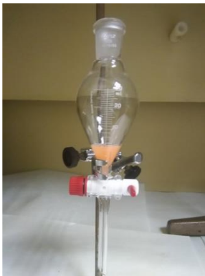
Figure 3.2.8. Decantation of the QDs after ligand exchange. Upper organic phase (toluene) and lower aqueous phase.
