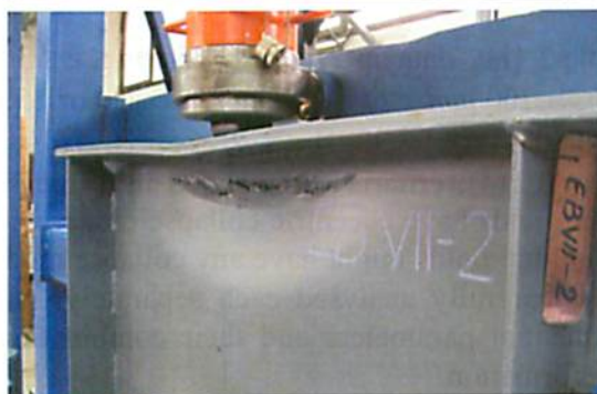
Figure 9. Centric collapse mode (t w = 5 mm, t f = 12 mm, e = 5 mm)
