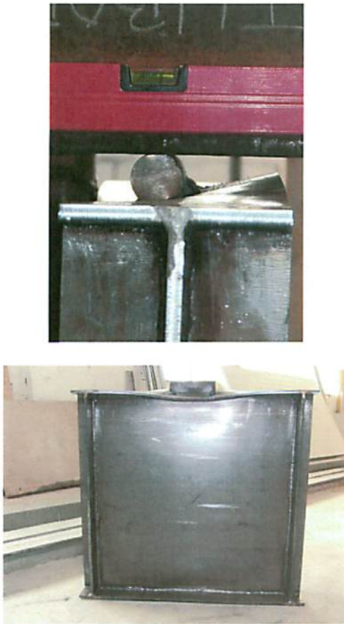
Fig. 10. Eccentric collapse mode observed in Spain corresponding to a = h_w = 700 mm, b_f = 150 mm, c = 150 mm, t_f = 10 mm, t_w = 10 mm and e = 15 mm.
