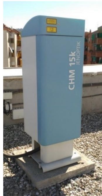
Figure 3.3. Ceilometer operated at UGR station.
