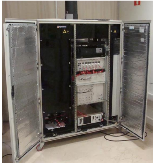
Figure 3.2. Raman lidar system operated at UGR station.
