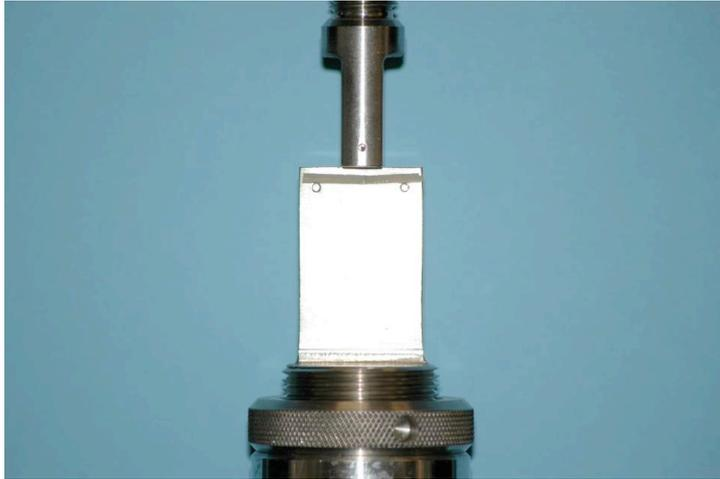
Figura 19. *Three-point-bending test.*
