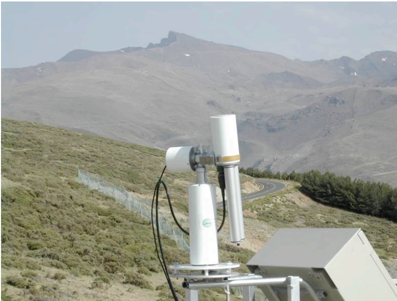
Figure 4.13. A Cimel CE 318 fielded in Sierra Nevada (Granada, Spain)
