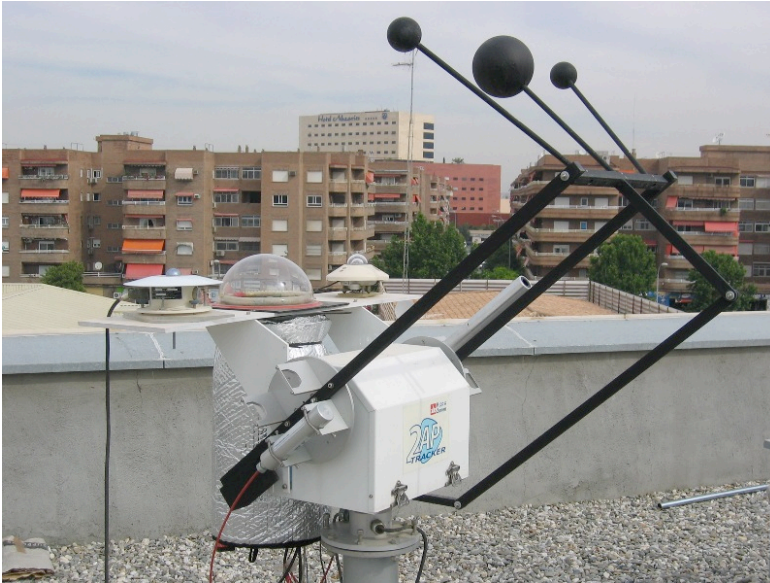
Figure 4.2. Final configuration of the All-Sky Imager placed in the Sun Tracker
