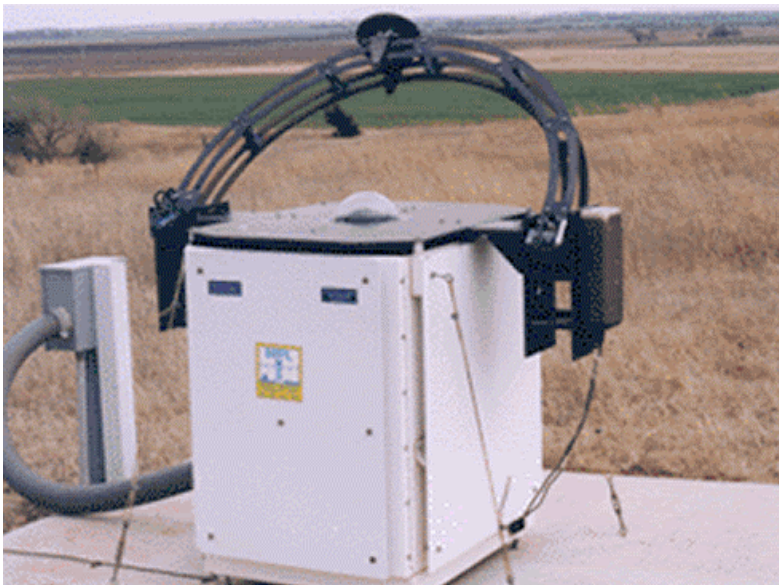
Figure 4.9. Day/Night WSI fielded at SGP CART site
