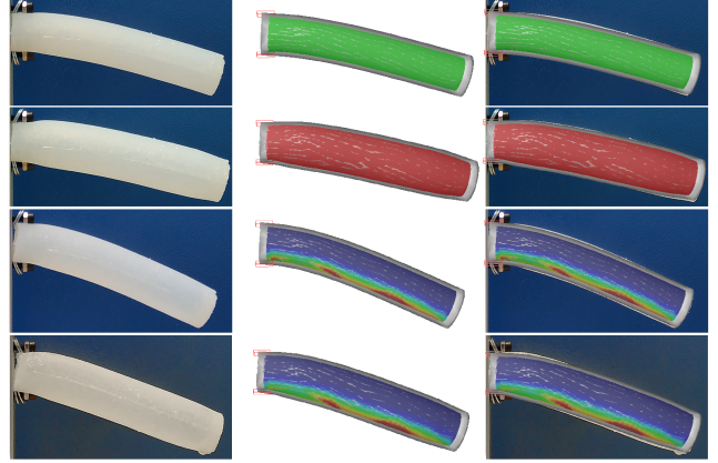
Fig. 4. Comparison of the fabricated silicone cylinder and the simulation of the same setup. From top to bottom, filled with air in rest state, inflated with 15 ml, filled with water in rest state and inflated with 15 ml.
