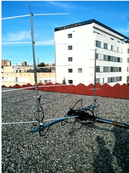
Figure 4.3 – X-Quad antennas mounted on the rotor
