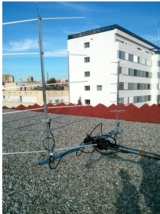
Figure 6.5 – X-Quad antennas mounted on the rotor
