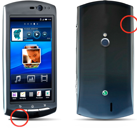
Figure 1.2: Example of smartphone embedding two microphones the location of which is marked with red circles. Front (left) and back (right) sides of the smartphone are drawn.
