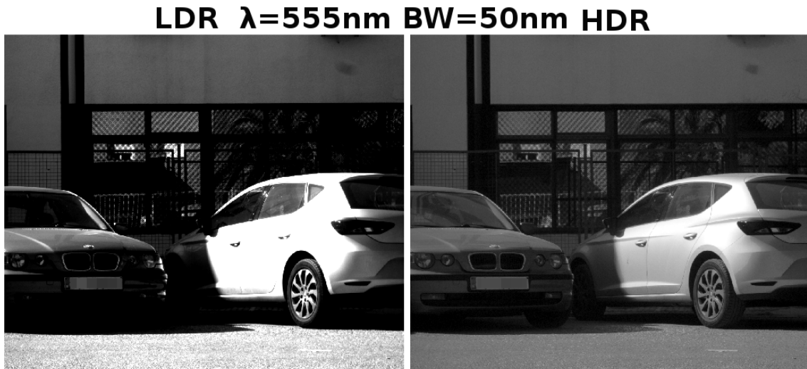
Figure 5-33: Grayscale images of scene 1 (see figure 5-31) captured at 555 nm with a bandwidth of 50 nm and polarization angle 0°. Left: LDR image. Right: tonemapped HDR image.
