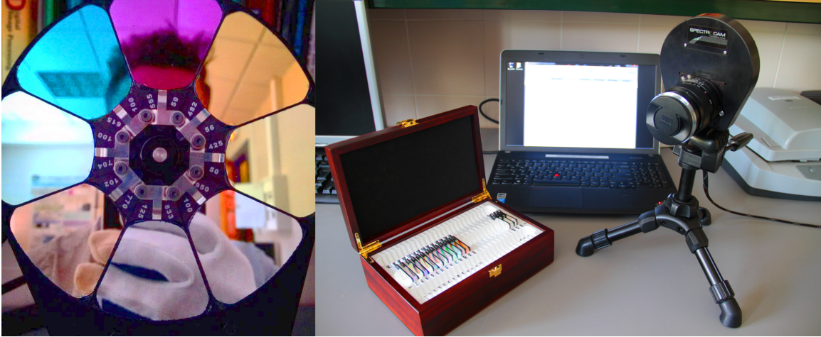
Figure 3-9: Pixelteq Spectrocam VIS-NIR . Left: 8-slots filter wheel. Right: camera with filter wheel attached, and 16 band-pass filters covering the visible and near infrared range of the spectrum [400nm, 1000nm].
