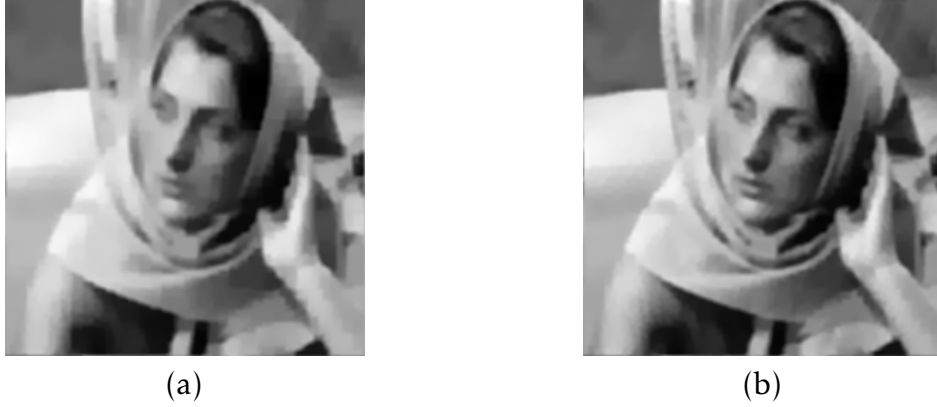
Figure 3.2: Joint estimation process. Observations have been simulated using Gaussian Blur of variance 3, zooming factor P=2 , Gaussian circulant Toeplitz measurement matrix with compression ratio R=0.8 , and additive noise of \text{SNR}=40\text{dB} . (a) First iteration estimate with \text{PSNR}=22.8\text{ dB} , (b) last iteration estimate with \text{PSNR}=23.9\text{ dB}
