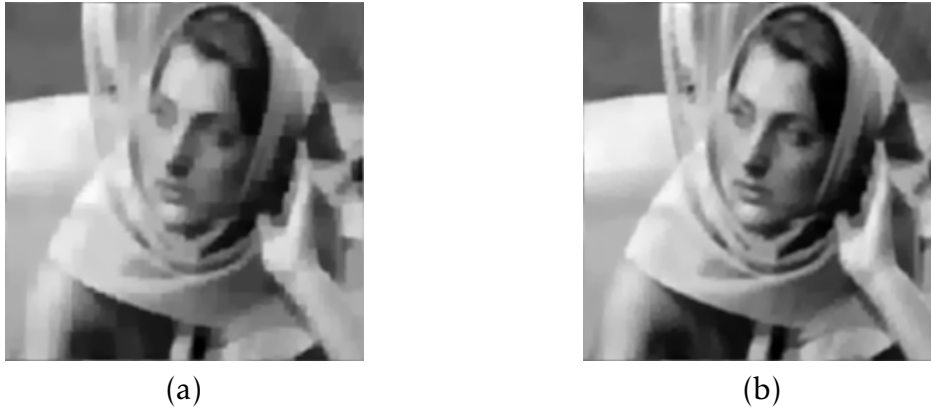
Figure 3.3: Joint estimation process. Observations have been simulated using Gaussian Blur of variance 3, zooming factor P=2 , Bernoulli circulant Toeplitz measurement matrix with compression ratio R=0.8 and additive noise of \text{SNR}=40\text{dB} . (a) First iteration estimate with \text{PSNR}=22.7\text{ dB} , (b) last iteration estimate with \text{PSNR}=23.9\text{ dB}
