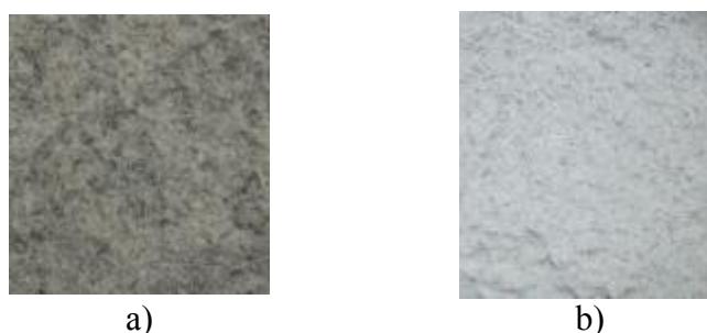
Figure 21. Ash photos of washed straw samples: a) at 550 °C; and b) at 1000 °C
