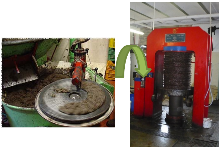
Figure 7. Traditional olive press with fibre discs.
