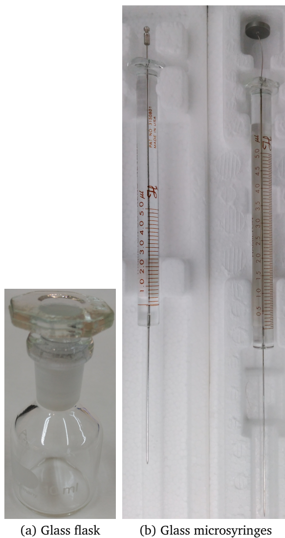
Figure 4.10: (a) Glass flasks and (b) glass microsyringes used with the organic spreading solvents, such as CHCl_3 and THF .
