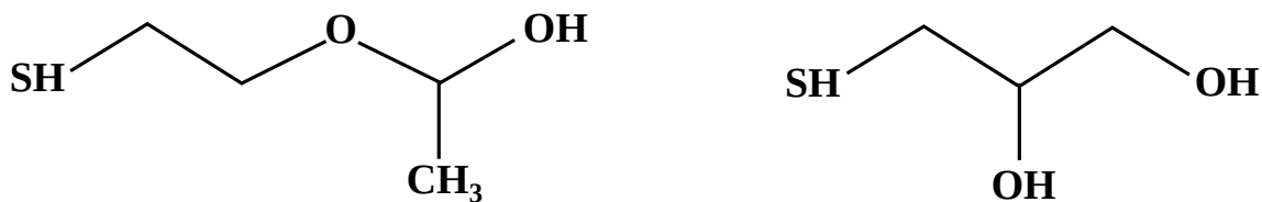
Figure 8.2: MEE (left) and MPD (right) capping ligands. The SH group is the anchor group at the gold nanoparticle surface.
