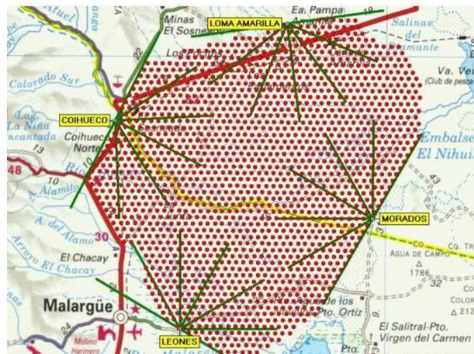
Figure 2.1: Map of the Pierre Auger Observatory. Red dots indicate SD detectors and green lines show the field of view of the FD telescopes.
