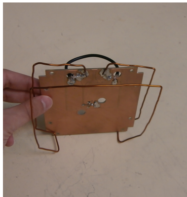
Figure 6.26 – Bodipole mounted with the coaxial balun
