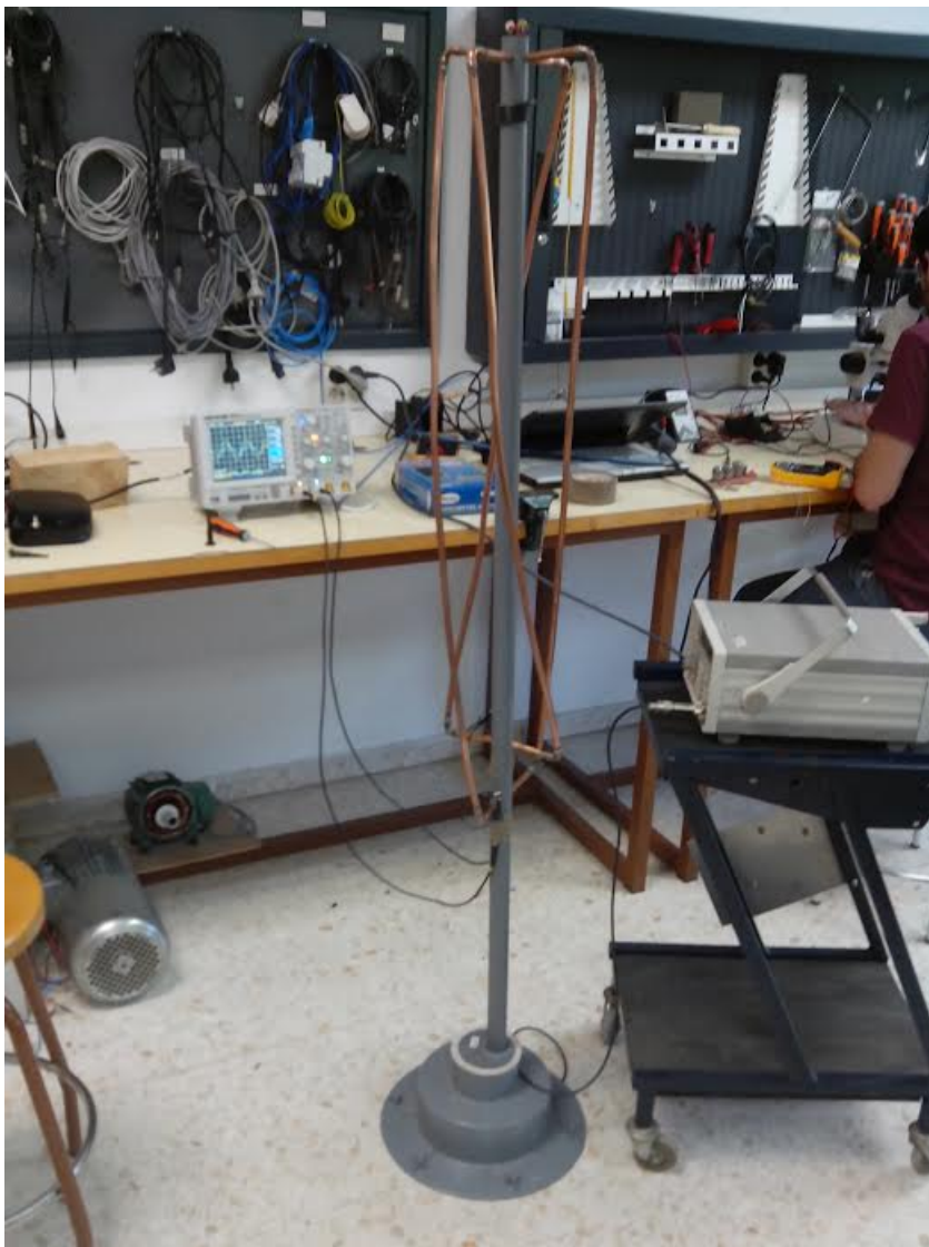
Figure 5.24 – Checking the polarization of the antenna.
