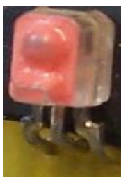
Figure 156. Picture of the covered photodetector. The pinkie film sensitive to oxygen is shown in the active face of this device.
