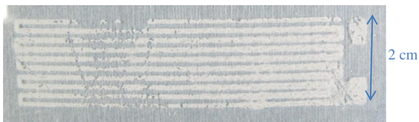
Figure 78. TME+NPG on PET substrate by flat screen printing.
