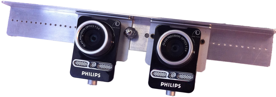
Figure 3.7: Stereo cameras set used for disparity computation. Typically, the separation between cameras is similar to the human eyes distance.
