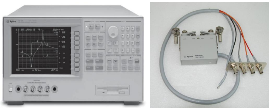
Figure 4: Impedance analyzer and connectors used to extract capacitance curves from the Pseudo-MOSFET samples.
