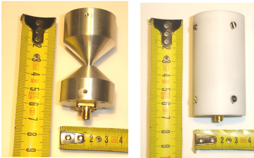
FIGURE 5.10: Wideband biconical antenna. Left: antenna assembly. Right: antenna with radome.
