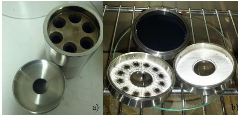
Figure 34. a) Section of the LPI-3 impactor used in this study; b) Quartz microfiber filters after testing
