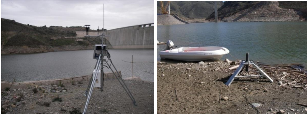
Figure 4.7 Photographs of the instruments used in the field study (a) Meteorological station at Location A (b) ADCP sensor fixed to tripod prior to deployment at Location C
