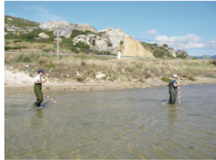
Measuring depth with leveled sticks
