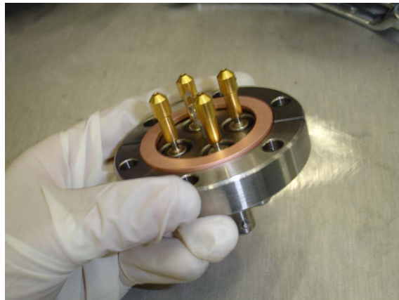
Figure 3.21: Feedthrough used for two of the level meters (each level meter uses two pins).
