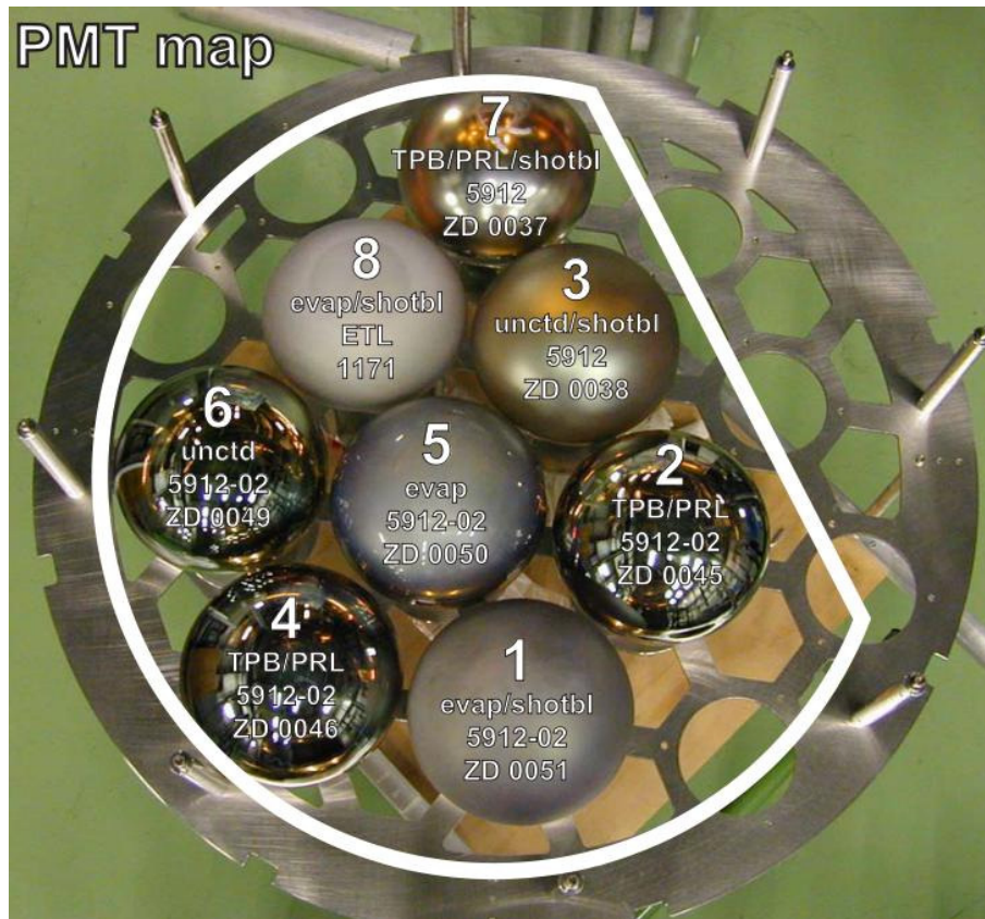
Figure 2.31: Positions of the PMTs during the first surface test in the ArDM experiment. The position of the field shaping rings is marked with a white line. The first line on every PMT refers to the coating procedure (see text) and if the window has been shotblasted. The second line is the PMT model and the third one the serial number used in our simulation.
