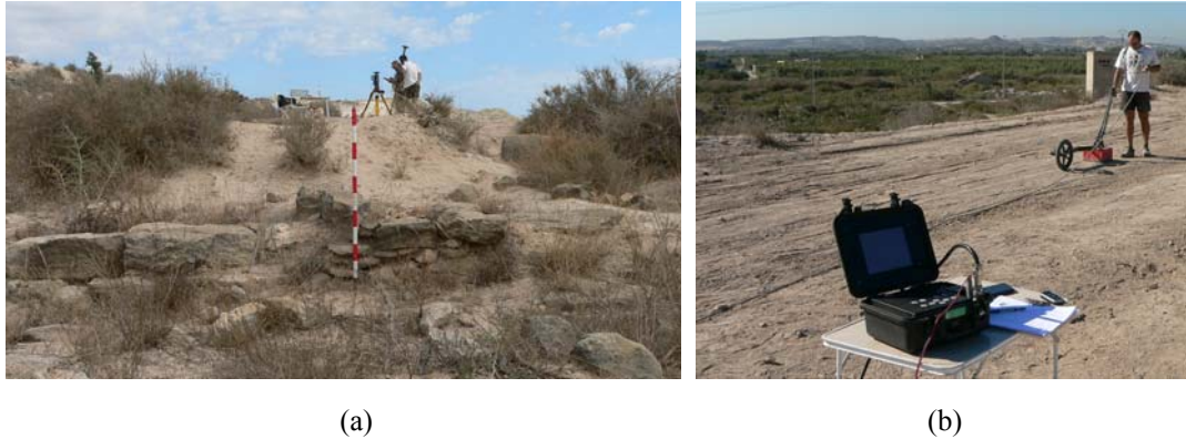
Figure 2. (a) Iberian structure excavated near the study area. (b) Basic GSSI equipment for data acquisition: a 400-MHz antenna with an odometer and recording unit attached to the back. A guideline at every 50 cm (profile separation) was used to place each profile.
