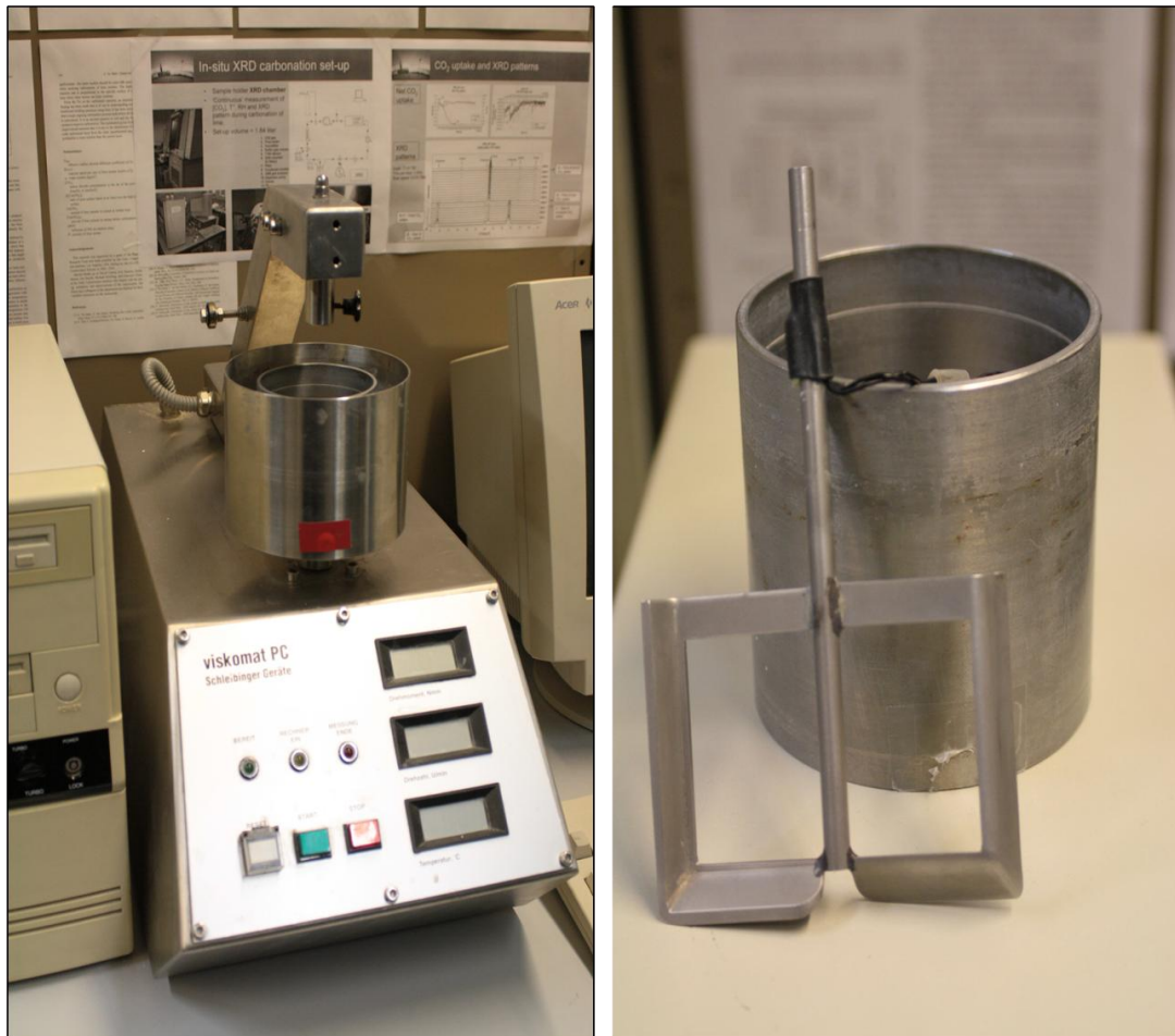
Figure 2 Photos of the Viskomat PC used (a) and geometry of the paddle (b).
