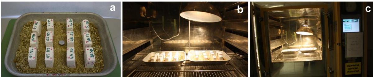
Figure 8 Durability study. (a): mortars samples placed in a tray over a sand layer; (b) and (c): interior of the environmental cabinet, where the samples were analysed.
