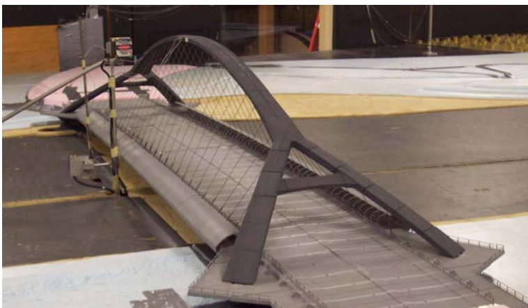
Figure 1.11: View of the 1:125 full aeroelastic model of the 3rd Millennium Bridge in the UWO, BLWT II Low Speed test section.
