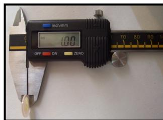
Fig.IV.D.3.-7-Electronic Digital Caliper
