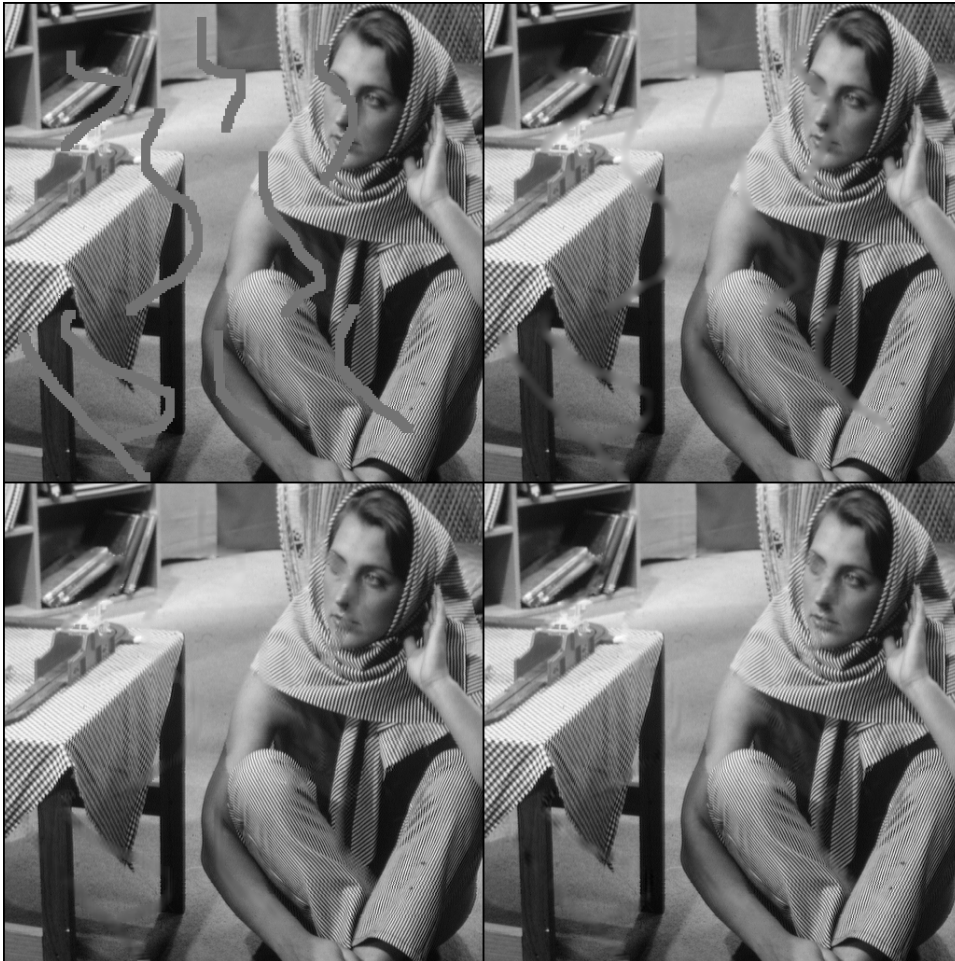
Figura 13.8: Top-left , Barbara image where value of missing pixels is the global mean of the observed ones (PSNR: 24,19 dB). Top-right , Fast-inpainting result (32,71 dB). Bottom - left , EM-inpainting result using 6-scale Curvelets and LDCT with block size 32 \times 32 (34,14 dB). Bottom-right , \ell_0 -GM result using 6-scale Curvelets (34,92 dB).
