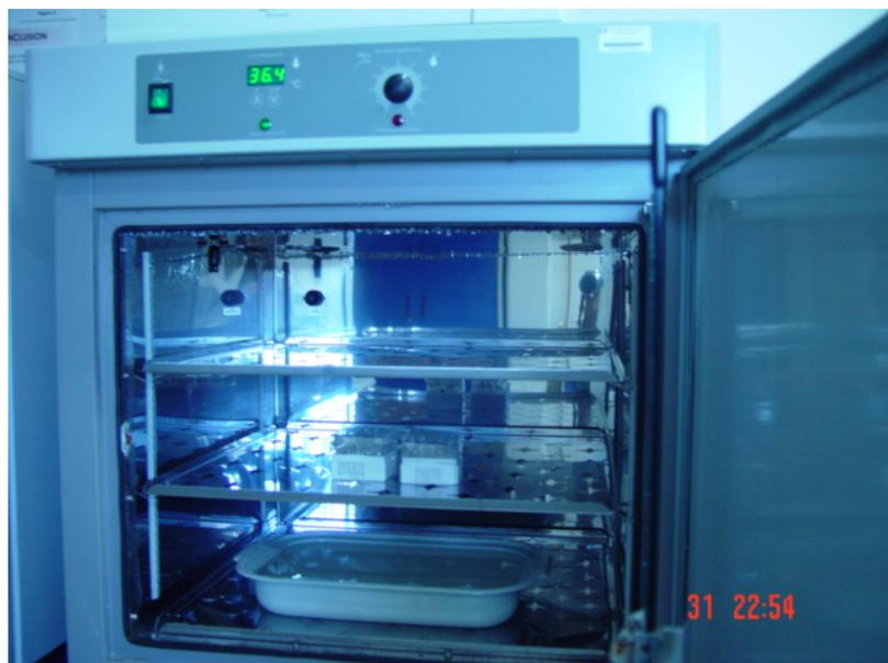
Figura 12. Incubadora Shel, Lab. VWR Scientific Products Modelo 1535.
